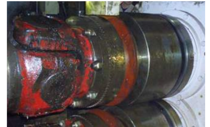
HYGUARD® safety coupling type HDW 300 with torque measurement system in a cold rolling mill after years of service
