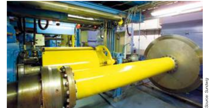
Curved-tooth coupling LBLKT 225, coiler drive in cold rolling mill
