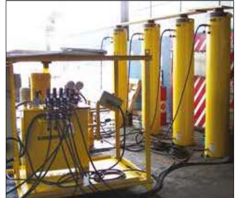
▲ Custom 500 ton double-acting cylinders with 1,83 m stroke for lifting electric rope shovels.
