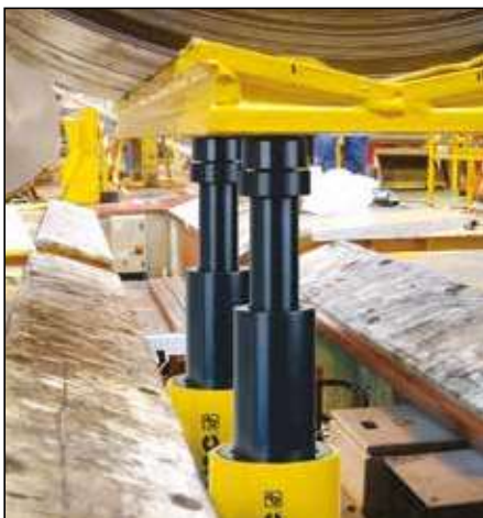
◀ The longer stroke length of telescopic cylinders will save you time and simplify projects by moving a load a greater distance and eliminating the use of temporary cribbing.
